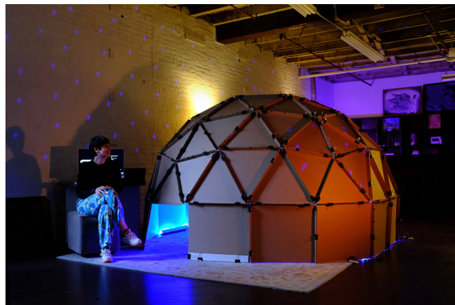
Figure 3: The geodesic dome built for Sensorium 1.2 made with cardboard and over one hundred paper clips.
